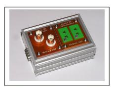
Supports modules specialized for signals typology, converts analog signals in digital form, memorie configurations and calibrations
