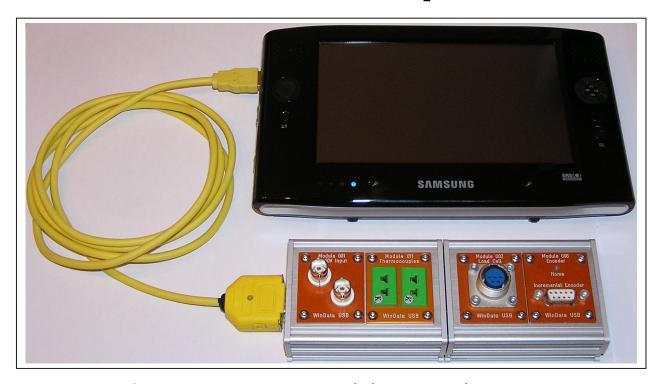
WinData USB system is composed by several acquisition units connected in sequence, each unit supports specific modules for connections to many transucer typology, the units chain is connected at an USB port of a PC using a small adapter. USB connection also supply the power for all components.
